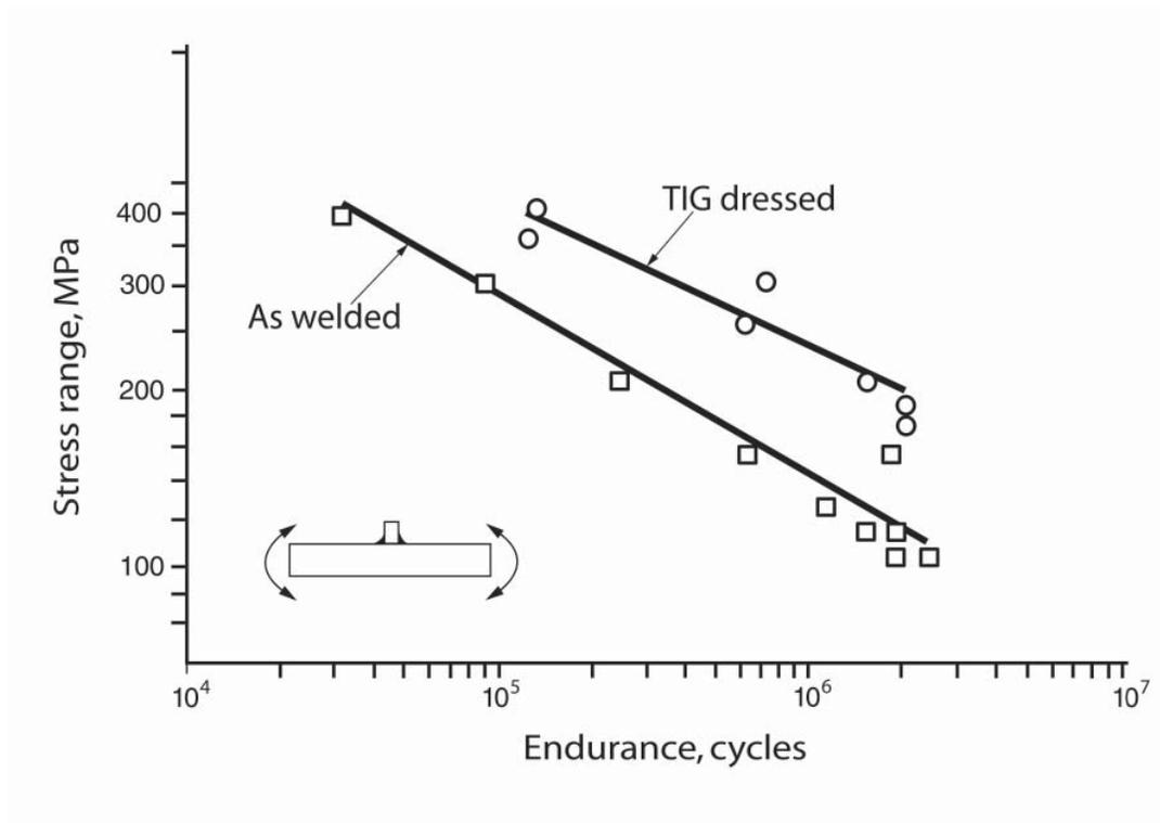
Figure 7 - Effects of TIG Re-melting
