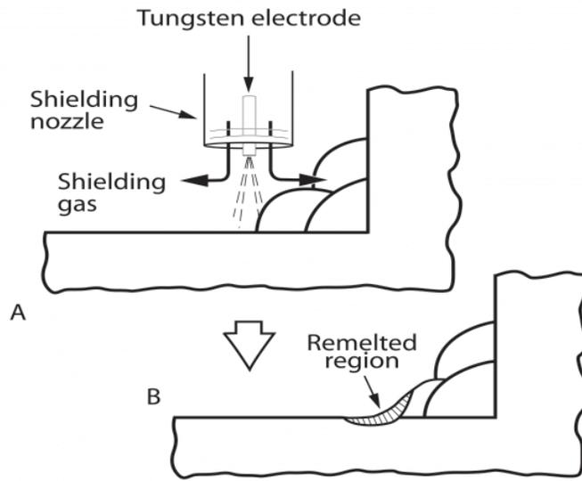
Figure 6 - TIG Re-melting
