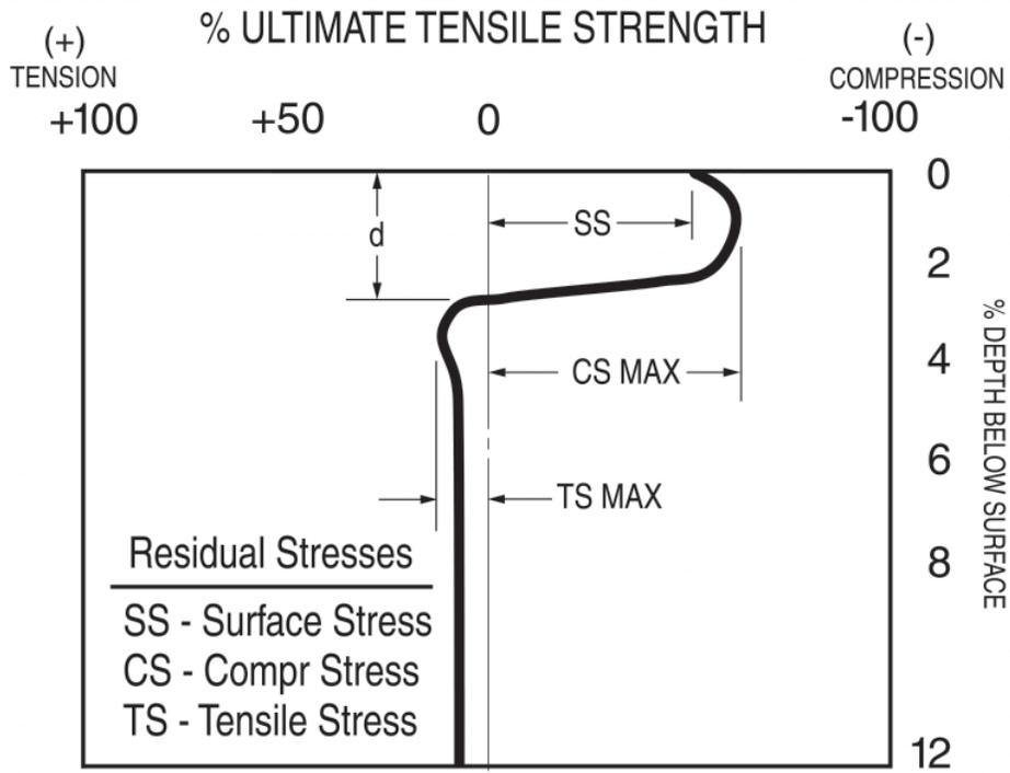
Figure 10 - Residual Stresses after Shot Peening
