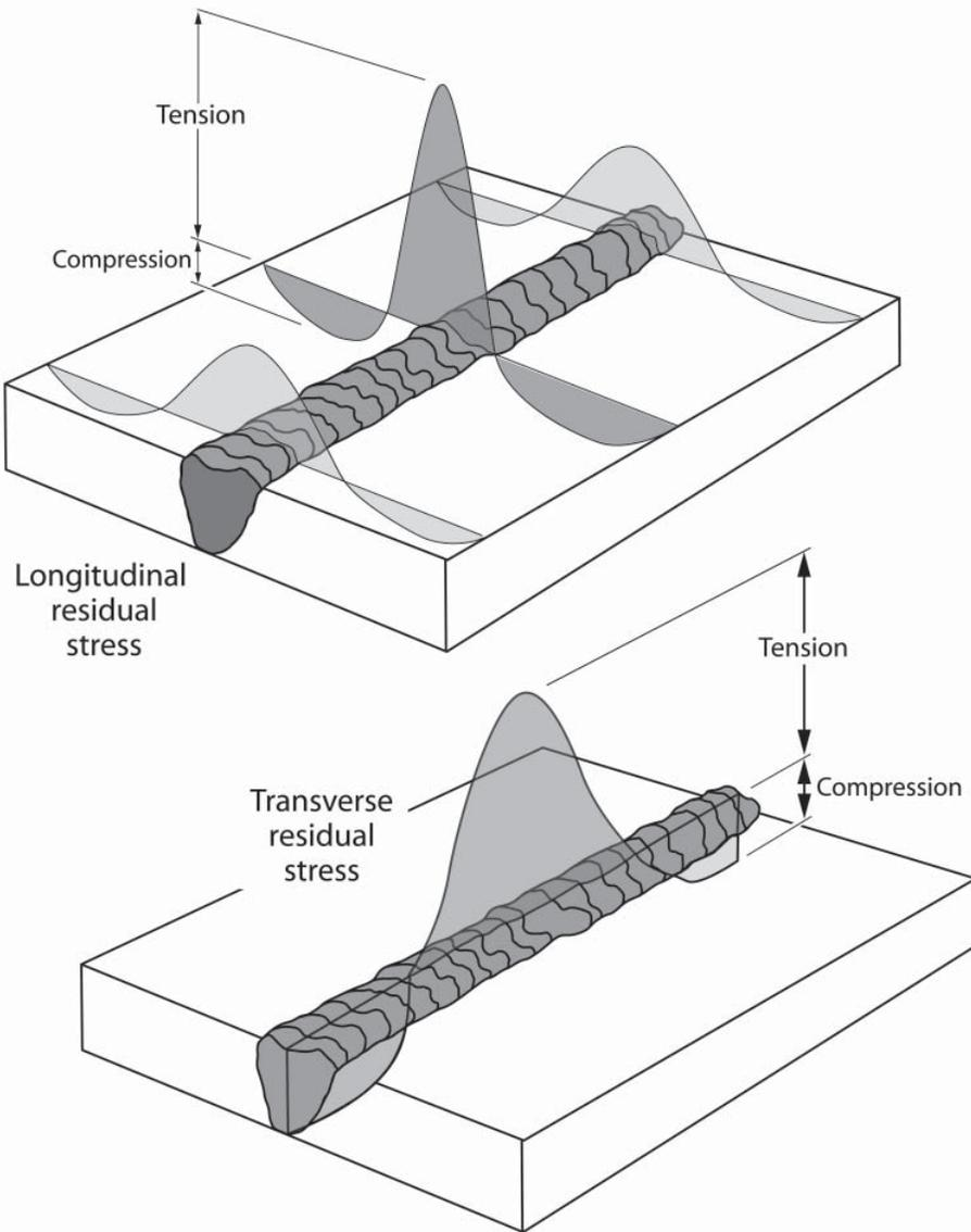
Figure 9 - Residual Stress Distribution after Welding
