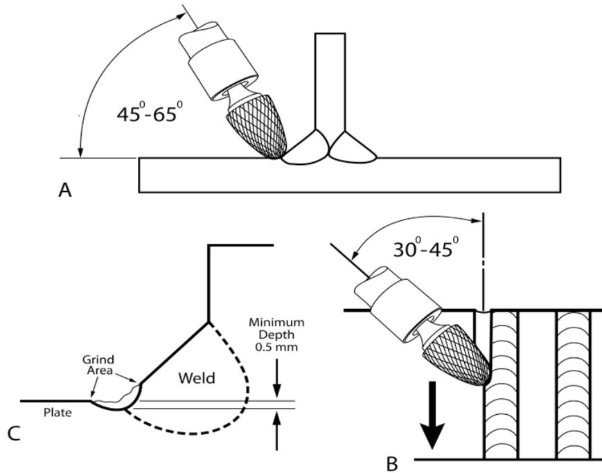
Figure 5 - Burr Grinding
