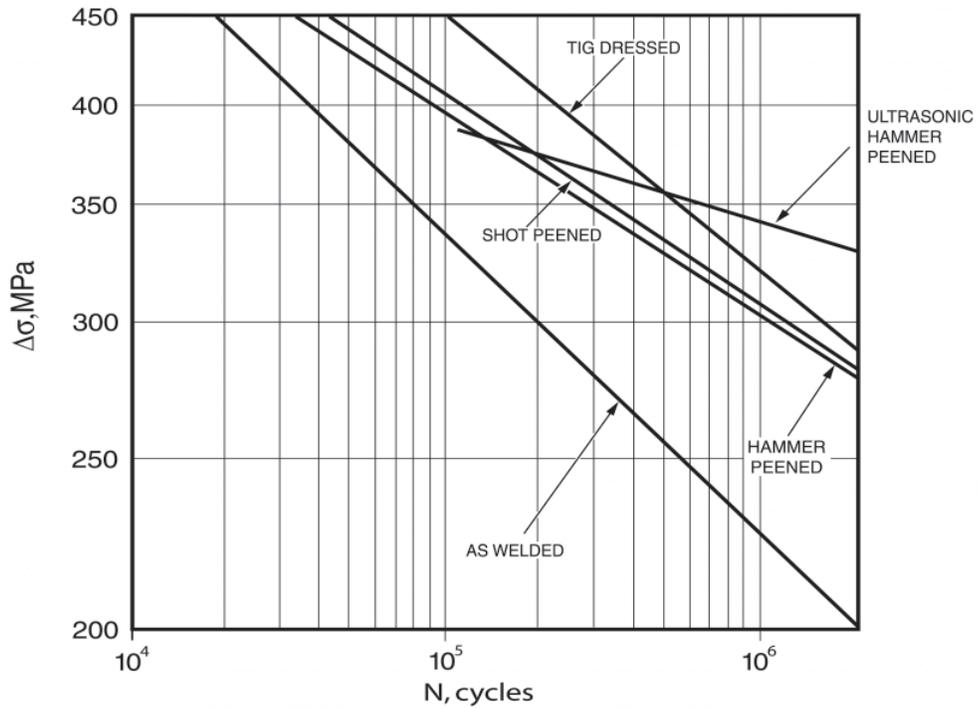
Figure 13 - Comparison of Effects - HSLA Steel
