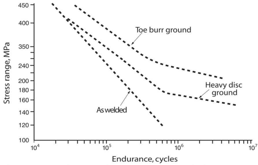
Figure 4 - Effects of Grinding
