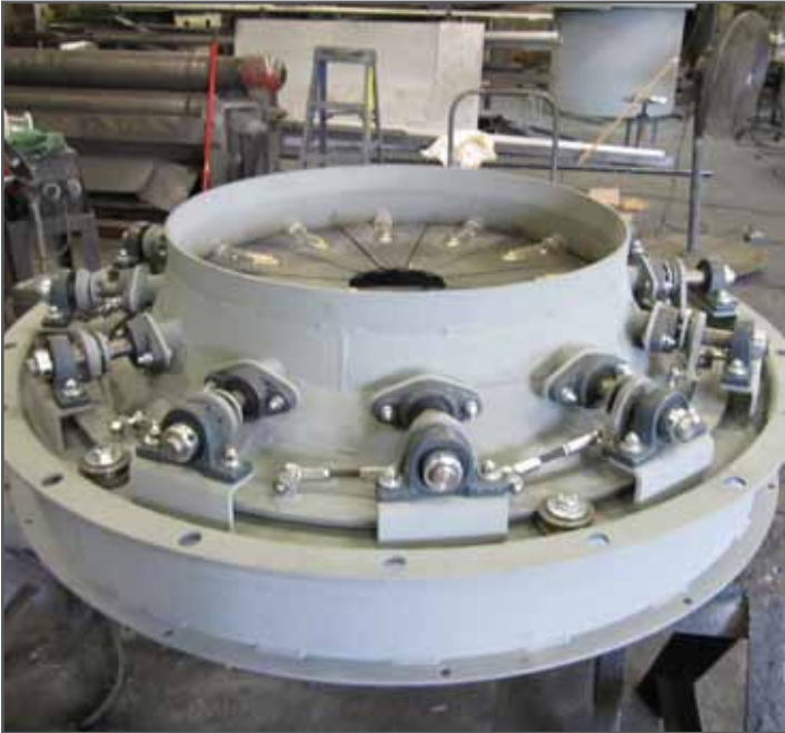
BURNER REGISTER DAMPER
