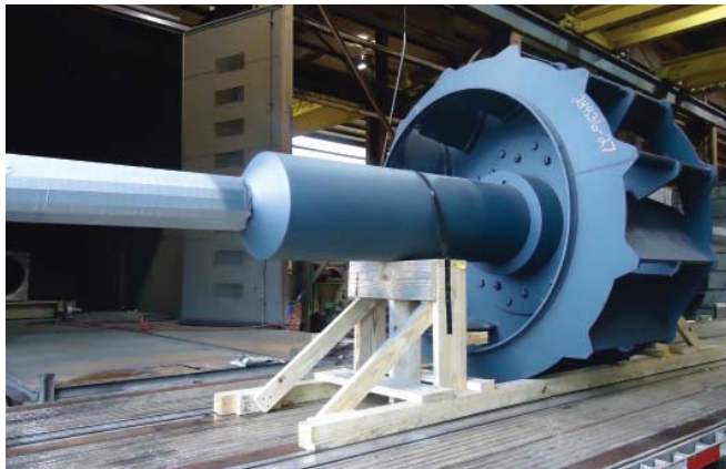
The paper mill ID fan was retrofitted with a radial-tip rotor at ProcessBarron headquarters in Pelham, Ala., and then installed in the existing fan casings at the mill.
